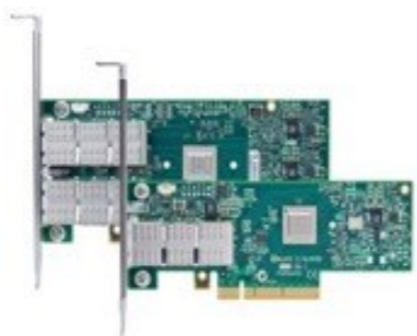
High Performance Interconnects – InfiniBand (DPU), Slingshot <1usec latency, 200-400Gbps Bandwidth>
